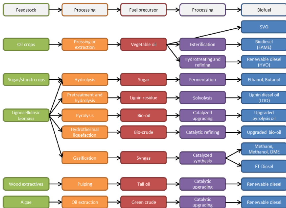
Figure 8. Overview of different feedstock conversion routes to marine biofuels including both conventional and advanced biofuels.
